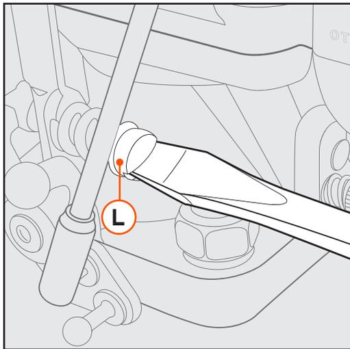
**B)** Now adjust the idle mixture (idle quality) using the idle needle screws (see J) with the engine at normal operating temperature, the air cleaner in place, the throttle fully closed and the choke fully open (see K). Turn the idle screws IN (clockwise) to provide a leaner mixture and OUT (counter-clockwise) to provide a richer mixture.
