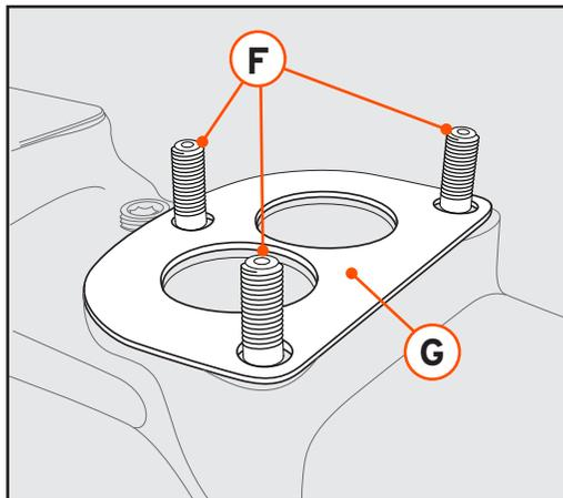
**NOTE:** Do not overtighten the mounting studs or bolts. Overtightening can result in damage to the manifold, manifold studs or carburetor base, that is not covered under warranty.
