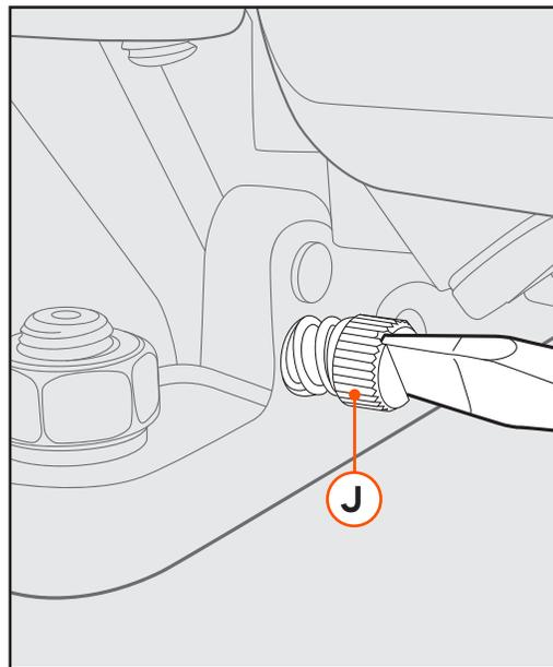
**NOTE:** If you have an engine vacuum gauge, set the idle screws to provide the highest and most steady manifold vacuum reading at idle.
